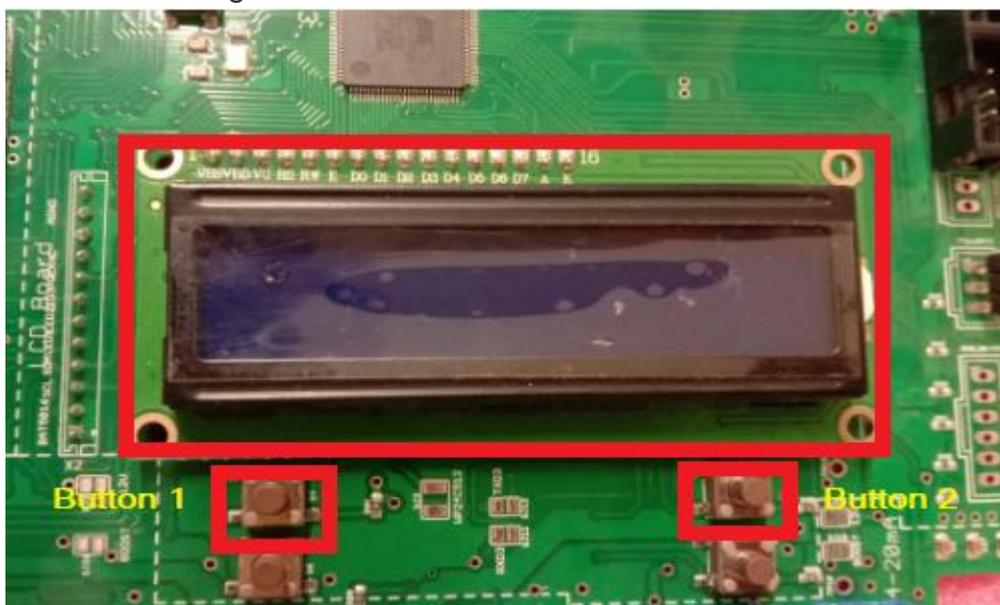
Fig 5: Internal LCD with Buttons
